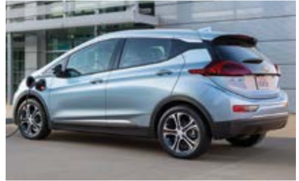
7.2 kW Level 2 charging enables refueling at the rate of 25 MPH. 50kW SAE Combo enables charging at 170 MPH.
